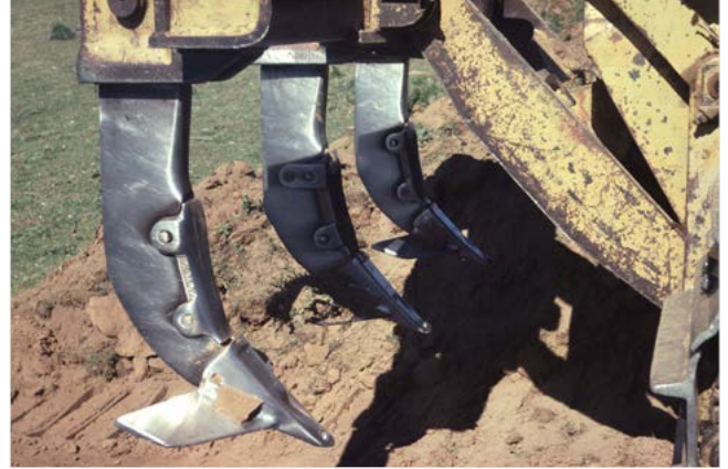
Figure 1: Ripping tines with winged tips on a Caterpillar D5 bulldozer used for warren ripping. Image: Brian Lukins
